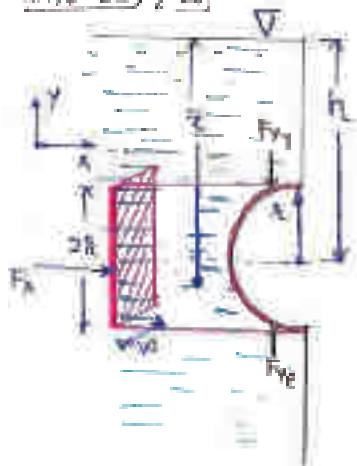
$$\begin{aligned} F_x &= \gamma A \bar{x} \\ &= (\rho g) [2\pi R w] [h] \end{aligned}$$
