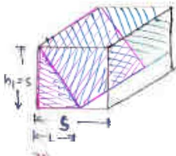
$$\text{Vol}^m \text{ spilled} = \frac{2}{3} (s^3)$$
