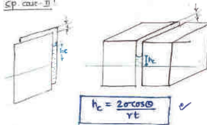
Note If  $h_c = 55 \text{ cm}$  ? It height is  $50 \text{ cm}$  then that is over flow
