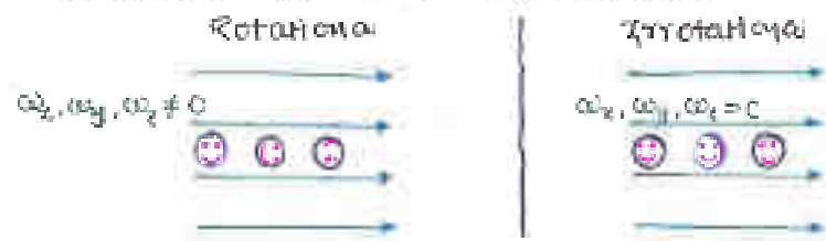
NOTE: ① Rotational is because of variation in shear i.e. difference in velocity of adjacent layer
