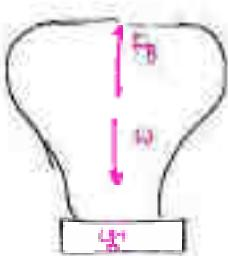
$$\begin{aligned} W_{(man+CH_4)} &= F_B (\text{air}) \\ mg + (\rho_{CH_4} g) V &= (\rho_{air} g) V \\ V &= \frac{95}{\rho_{air} - \rho_{CH_4}} = \frac{95}{(1.25 - 0.75)} \\ V &= 150 \text{ m}^3 \end{aligned}$$
